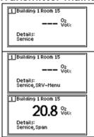
For a number of transmitters with an analogue interface, the current level indicates to the GMA200 that maintenance work is being carried out on the transmitter. In this case, no measured value is displayed and, depending on the screen, "SRV" is displayed at gas type and "Maintenance" at detail.
