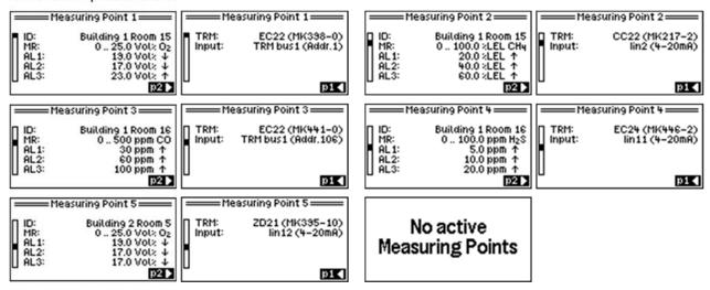
Note: Minor adjustments can be made as explained in section 4.5.3 "Service menu / "Measuring Points". More complex changes, such as adding or removing measuring points, are only possible using the configuration software GMA200Config.
