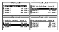
With "Alarm Limits", the limit values for Alarm 1, Alarm 2 and Alarm 3 can be changed within the measuring range after the measuring point has been selected. If the alarm threshold is set to 0.0 (zero), the alarm is switched off.
