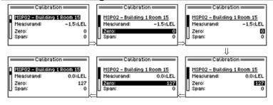
The measured value of the GMA may show small deviations compared to the current signal of a transmitter with analogue interface. With the "Calibration" these small deviations can be compensated.
