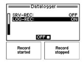
With "SRV-REC" the data recording for service purposes on the microSD card can be started or stopped for a maximum of 8 hours. This data recording for Service purposes works even if the GMA has no data logger. (file name: \*S.txt)
