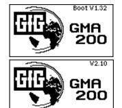
At system start-up the GfG logo, the device name and first the version number of the bootloader and then the version number of the mainboard firmware is displayed.
