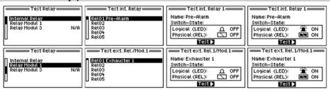
With relay "Test" the switching of internal relays of the GMA200 and of relays on external relay modules can be tested.
